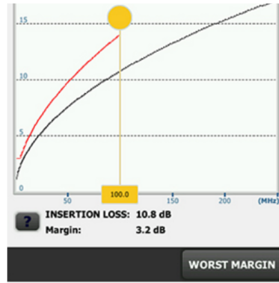
Figure 2. Measured Insertion Loss and limit for 450 foot Type 734 cable.
